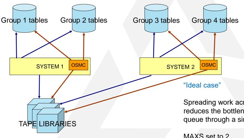
Spreading work across multiple OAM's / OSMC's reduces the bottleneck of a single input work queue through a single address space.
